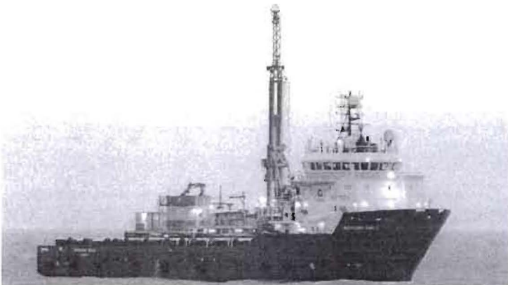
Subsurface data for tunnel design was collected in 2019 from the Highland Eagle, a drilling vessel supporting the required geotechnical work for this effort.
